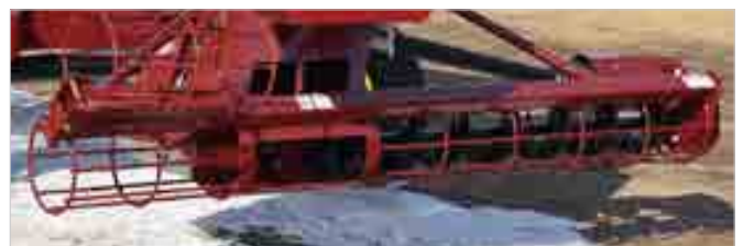
9" CROSS AUGER WITH CONTINUOUS FLIGHTING
