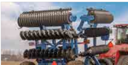
DOUBLE V BLADES NOTCHED FRONT, SMOOTH BACK
